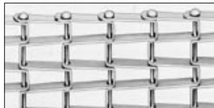
(D) Flat Wire. 1/2" x 1" grid, 3/8" high x 0.046" thick flat wire with connecting rods on 1" pitch.
