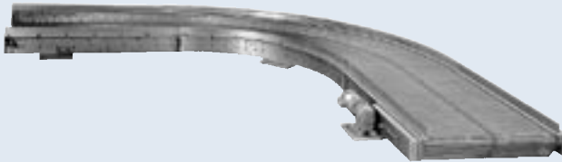
Serial No. 83241: Combination straight & turn wire belt conveyor, using rod type belt with mesh overlay in a snack food application.
