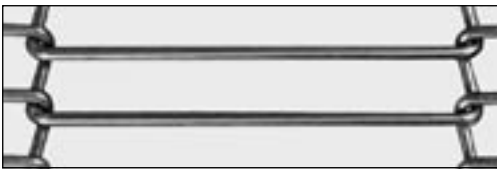
(A) Wire Loop 3/8" pitch, 0.082" wire, approx. 2-1/2" wide loops.
